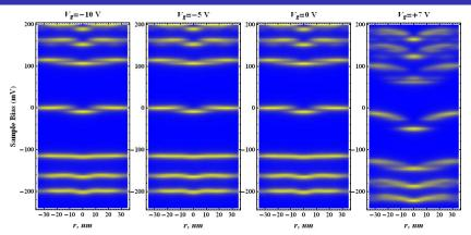
Theory: The local density of states plotted at four values of gate voltage and B = 10T - Sobol et al., Phys. Rev. B 94 (2016). The strength of the impurity depends on the occupation of Landau-levels which can be controlled by a gate voltage.
