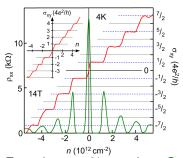
Experiment: Novoselov, Geim et al., Nature 438, 197 (2005). Kim, Stormer, et al., Nature 438, 201 (2005). Hall conductivity  $\sigma_{xy}$  and longitudinal resistivity  $\rho_{xx}$  of graphene as a function of their concentration at B =14T.
