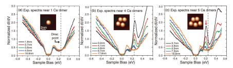
Spectra  $dI/dV \sim \rho(E=eV,r)$  at different distances from the center of Ca dimer clusters (i.e., artificial nuclei) as functions of a simple bias V(meV). For free massless Dirac fermions  $\rho(E) = \frac{2|E|}{\pi(\hbar v_F)^2}$  Experiment: Y. Wang, et al., Science 340, 734 (2013).
