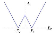
The band gap  $\Delta$  as a function of the electric field  $E_z$ . The gap is open for  $E_z \neq \pm E_c$ , where silicene is an insulator. It is a topological insulator for  $|E_z| < E_c$  (with edge states) and a band insulator for  $|E_z| > E_c$ .
