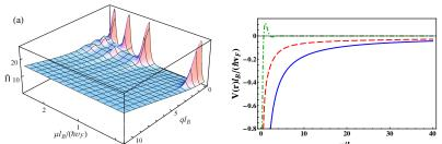
Polarization function as a function of the chemical potential and the wave vector (left panel) and the Coulomb potential (right panel).
