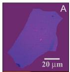
Photograph in normal white light of multilayer graphene flake K. Novoselov *et al.*, Science **306**, 666 (2004)
