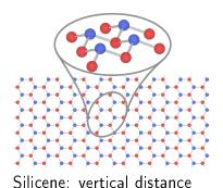
between sublattices  $2d \approx 0.46$  Å. Lattice constant a = 3.87 Å. 2D sheets of Ge, Sn, P and Pb atoms (the materials germanene, stanene and phosphorene).
