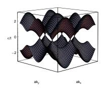
Two bands touch each other and cross the Fermi level in six K points located at the corners of the hexagonal 2D Brillouin zone.
